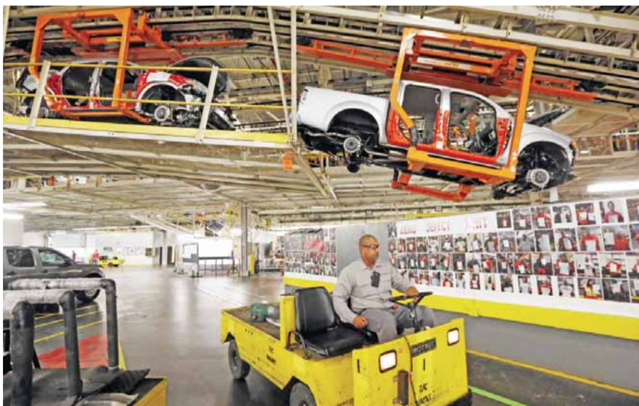
CANTON: Vehicles are suspended above other installation stations as they are moved along the assembly line at the Nissan Canton Vehicle Assembly Plant in Canton, Mississippi. — AP
