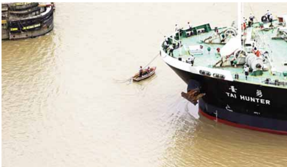
Two canal workers on a small rowboat catch a line from a massive cargo ship as it prepares to enter the Pedro Miguel locks in Panama City.
