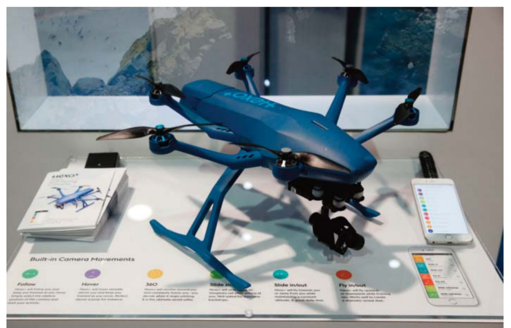
The Hexo+ Your Self-Flying Camera drone is on display at the Hexo+ booth during CES International on Jan 7, 2016. The fully autonomous drone has no controller. Using a smart phone app, the user selects how and from what angle you want the drone to take video of you and it will automatically follow you around with its camera.
