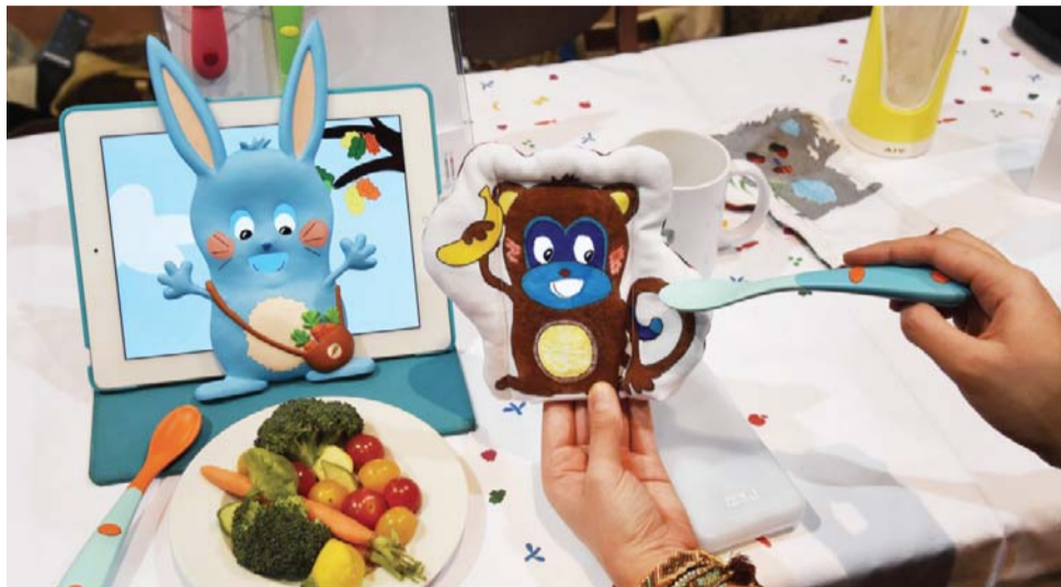
Slow Control's Yum & Done, the first smart spoon and a cuddly toy to help make kids eat their vegetables, is displayed. A button on the Bluetooth-enabled spoon activates an app on a smartphone or tablet that is covered by a cuddly toy to keep a child's attention while being fed from the spoon.
