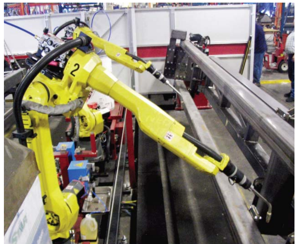
Articulated welding robots used in a factory, a type of industrial robots.
