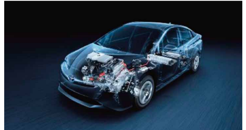
Hybrid system combining a 1.8-liter engine and electric motor delivers outstanding fuel economy of 40.8 km/litre which is more than 20 percent better compared to the previous model
