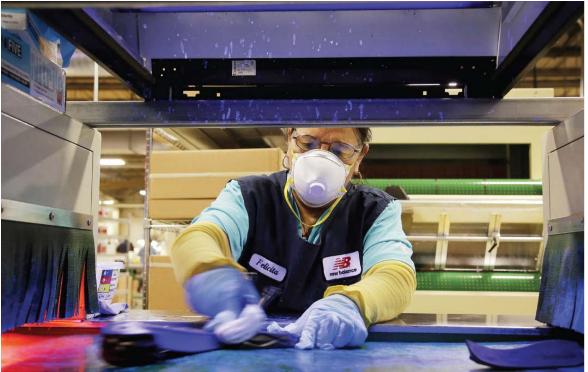
BOSTON: Primer is applied to the midsole of a military tested New Balance 950v2 sneaker under ultraviolet light before the outsole is attached at one of company's manufacturing facilities in Boston. The Institute for Supply Management, a US trade group of purchasing managers, issued its index of manufacturing activity for January. — AP
