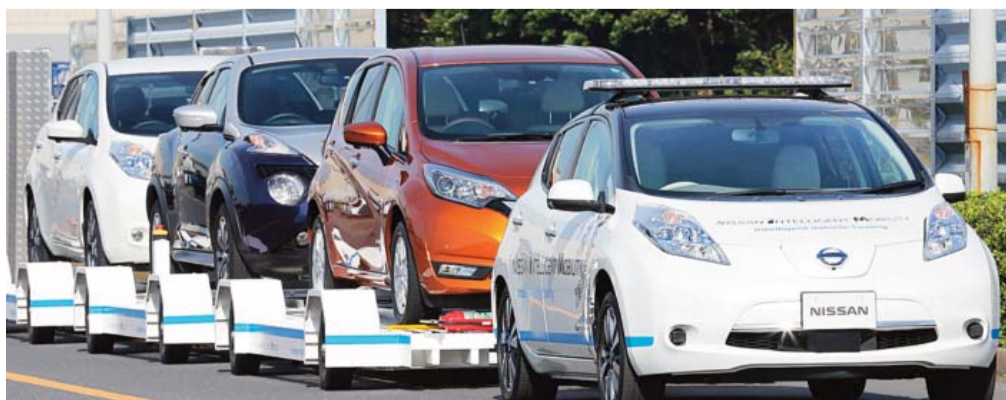
YOKOHAMA: Nissan Motor Co's "Leaf", with no one inside, pulls a trailer with three other Leafs on it, during a demonstration of the automaker's Intelligent Vehicle Towing system at Nissan Oppama plant. — AP
