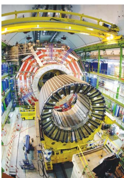
GENEVA: In this March 22, 2007 file photo, the magnet core of the world's largest superconducting solenoid magnet (CMS, Compact Muon Solenoid) at the European Organization for Nuclear Research (CERN)'s Large Hadron Collider (LHC) particle accelerator. — AP
