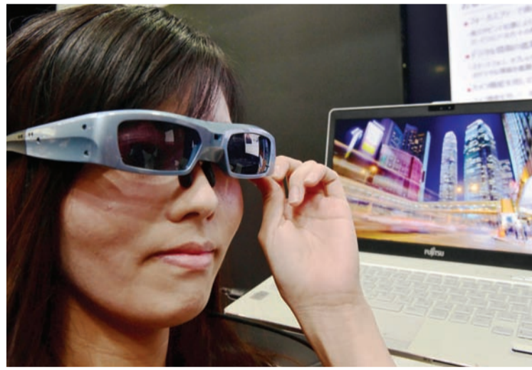
CHIBA: An employee of Japan's computer giant Fujitsu demonstrates a prototype of the "Retissa" retinal imaging eyewear - which can project digital images onto the user's retina using laser beams for low vision patients. — AFP
