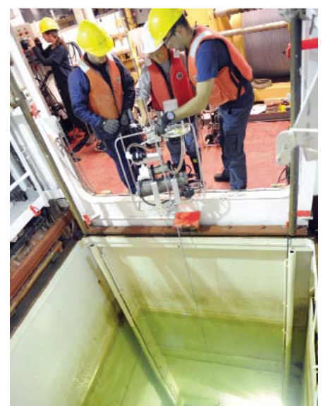
ARCTIC OCEAN, at sea: Members of the Canadian Coast Guard assigned to the CCGS Amundsen, assist scientists to deploy a pump through the hull of the ship.
