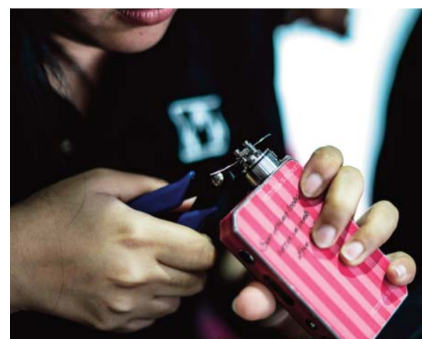
A worker inspecting a coil, the metal heating element in an e-cigarette that produces vapor from e-juices.
