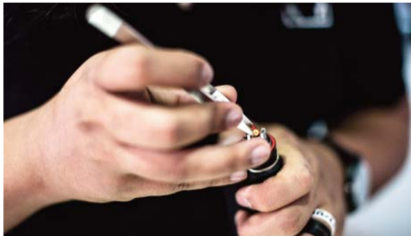
A worker inspecting a coil, the metal heating element in an e-cigarette.
